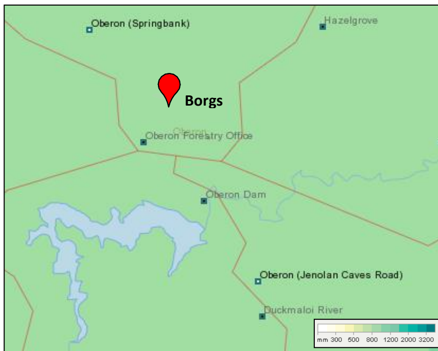
Figure 9.3. Location of pluviograph stations around the Borgs site. The uniform background colour indicates all stations are within the same zone of average annual rainfall around 800mm/year.
